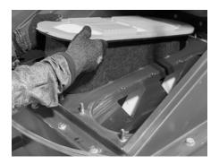
Grasp flange sides along edges and lift the old filter out.
