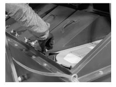
Remove filter retainer by unscrewing wing nuts and lifting retainer out.
